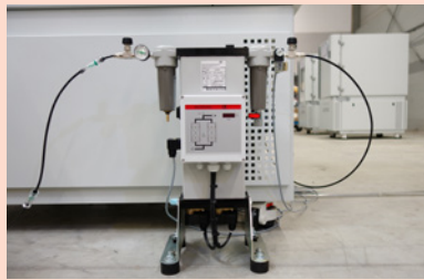
Compressed Air Dryer
