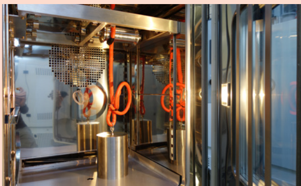
Cold Bend Cables Testing
