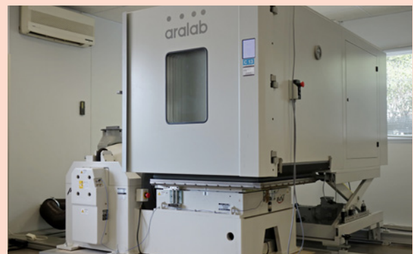
Shaker Integrations for vibration testing
